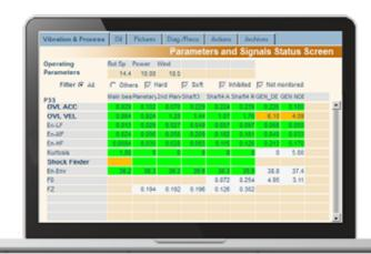
Defect Detection Grid (2DG) as presented to the expert in ONEPROD NEST Analyst software
